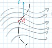
$$I = \int_{C} d\overline{\ell} \cdot (\overline{K} \times \hat{n}) = \int_{C} \overline{K} \cdot (\overline{n} \times d\overline{\ell})$$
