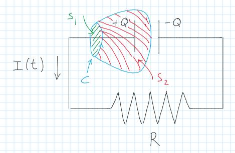
Now one can apply the integral form of Ampere's law without the displacement current to the surface S\_1 bound by the oriented path C. One finds as expected
