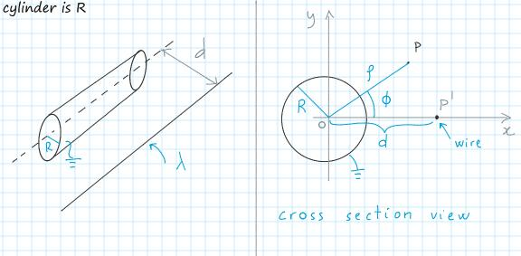
Part c) by using the result of part b, find out the potential in the case in which the infinite cylinder is isolated and is placed between two infinite straight uniformly charged wires. The two wires carry the same amount of charge per unit length, but the charges on the two wires have opposite sign.
