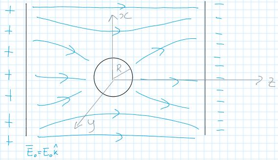
We can add an image dipole (in the space occupied by the sphere) to the potential responsible for the contact field. This combination solves the Laplace equation because each one of these two potential solves separately the Laplace equation.
