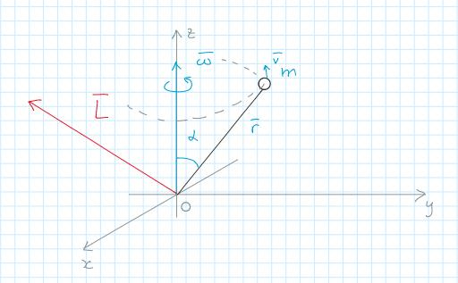
The direction of the angular momentum changes in time, so that there is a torque applied on the bar.
