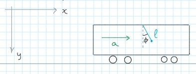
$$\overline{r} = (x, y) = (l \sin \phi + \frac{1}{2}at^2 + v_0t + x_0, l \cos \phi)$$
