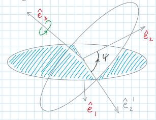
The angles  $\Phi$   $\theta$  and  $\psi$  are called Euler's angles. They specify the rigid body orientation with respect to the fixed space frame.
