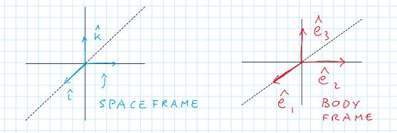
Begin from a situation in which the two frames coincide, with k and e\_3 in the same direction, and j and e\_2 pointing in the same direction.
