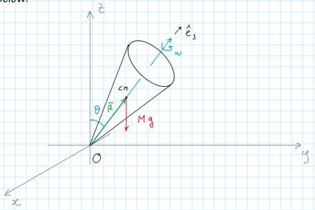
The inertia tensor calculated with respect to a frame centered in O, with the z axis along the axis of rotation of the cone is diagonal, because the axis of rotation is one of the principal axes of the object
