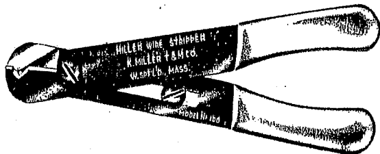
FIGURE 14-3(a) Miller Wire Stripper
