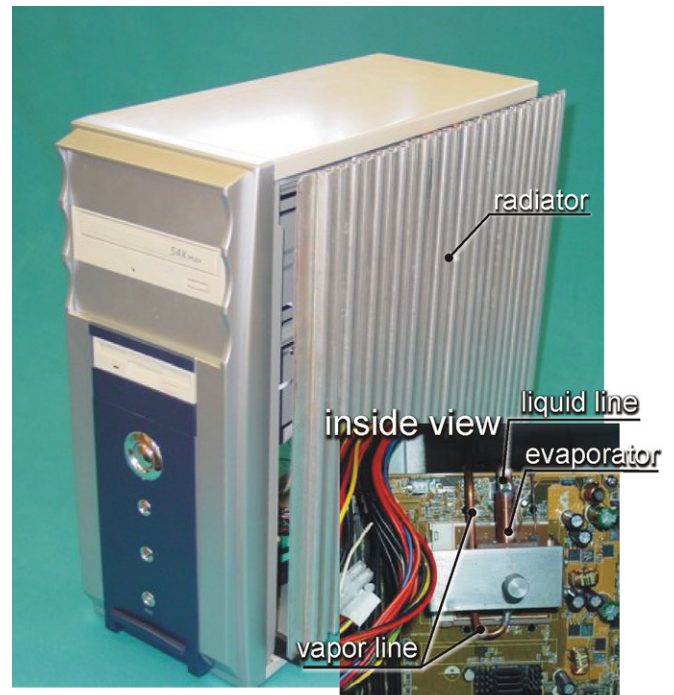
Fig. 5. General view of the cooling system CS #2 in the DC structure.
