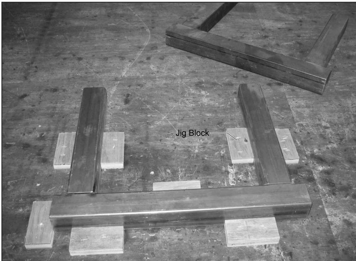
Jig Blocks in Use
