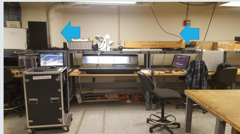
The initial setups of the entire system. Qlab on the right sends cue commands to GrandMA that is connected here with the MA VPU on the left where the console communicates with the video units.
