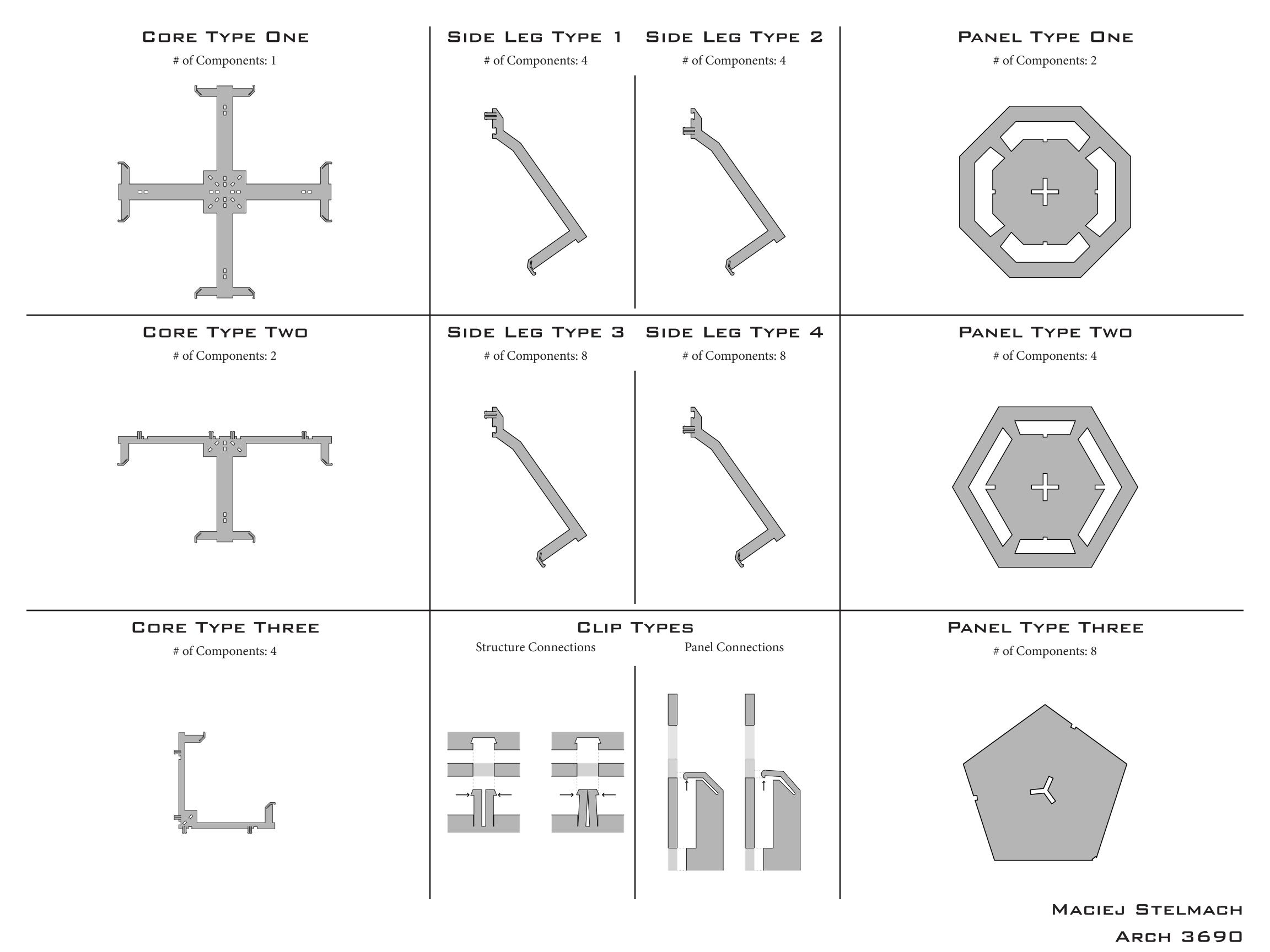
Side Legs Type One and Type Two are connected to each other through the Core Type One openings.
