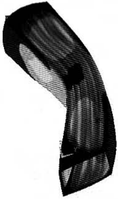
2.31. The FEM analysis for the fabric envelope of "Dynaform," BMW Pavilion at the IAA'01 Auto Show in Frankfurt, Germany, architects Bernhard Franken and ABB Architekten.
