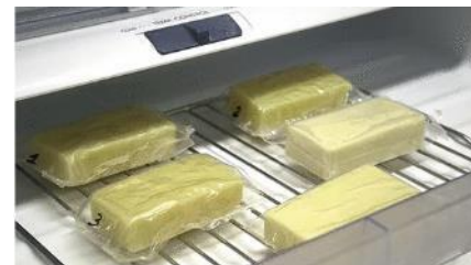
Edible plastic film made from the milk protein casein Source: Headline Science/American Chemical Society
