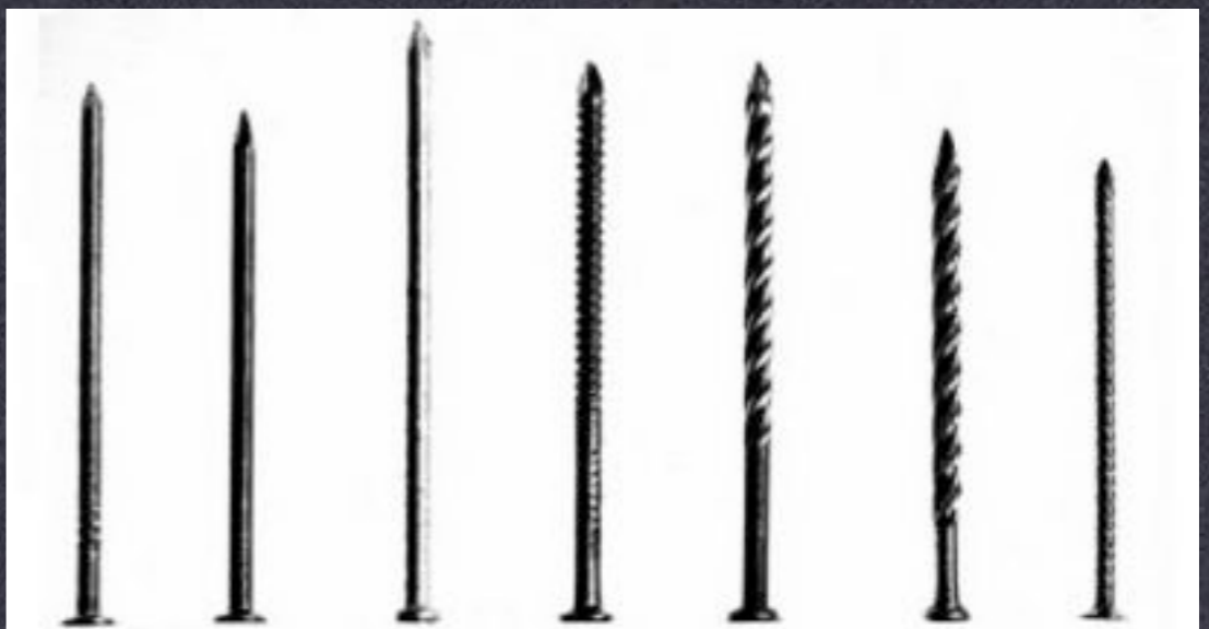
Various types of nails: (left to right) bright smooth wire nail, cement coated, zinc-coated, annularly threaded, helically threaded, helically threaded and barbed, and barbed.
