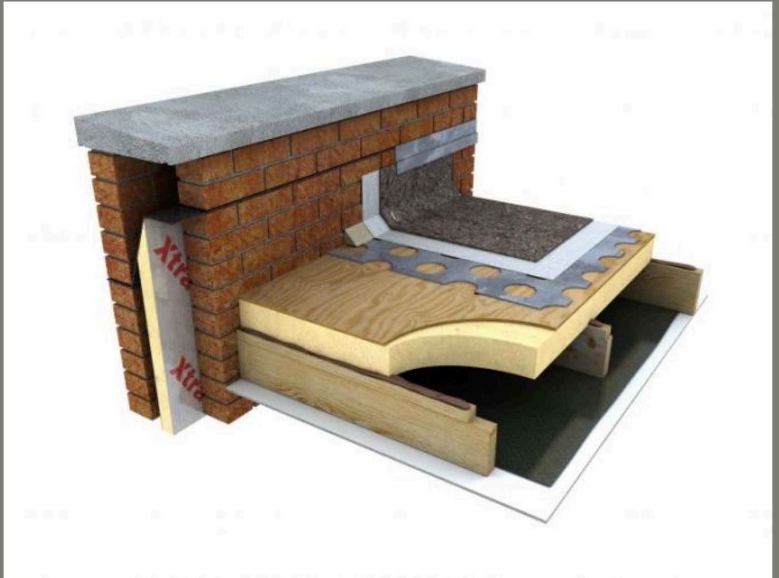
ROOF CONSTRUCTION AT BRICK PARAPET
