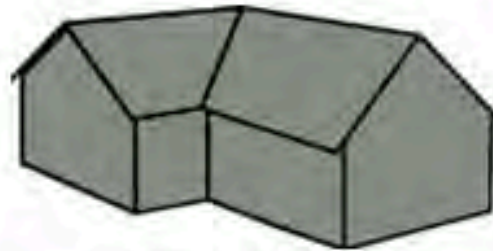
Cross Gabled Roof
