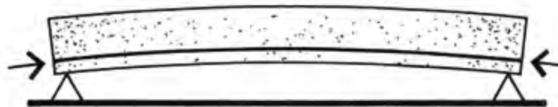
When a concrete beam is prestressed, all the concrete acts in compression. The off-center location of the prestressing steel causes a camber in the beam
