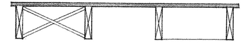
Bridging consists of wood or metal crossbracing or full-depth blocking between each joist at 8' (2440) intervals. Bridging may be required by some building codes if the joist depth is 6 or more times its thickness. However, it is usually not necessary if the joist ends are supported laterally against rotation and their top compression edges are restrained by sheathing or subflooring.
