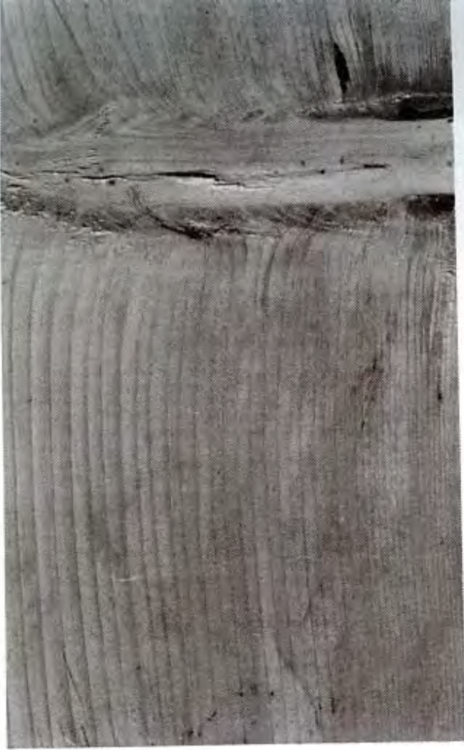
Knot: cut longitudinally
