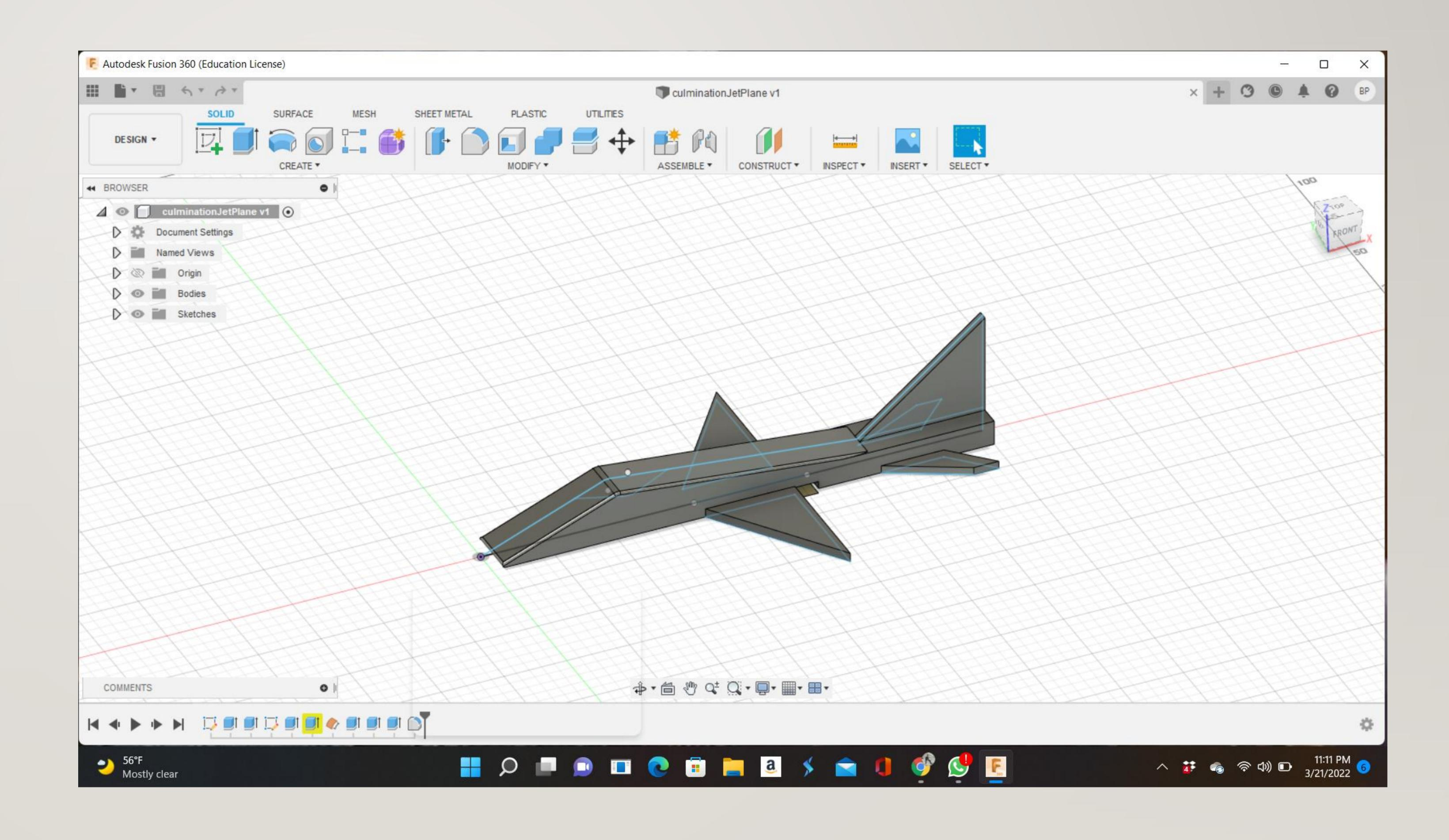
This is my Jet Plane after many changes, I used the canvas as a blueprint and built the entire jet plane. The wings, the front nose, the entire body were all different bodies put together to make one.
