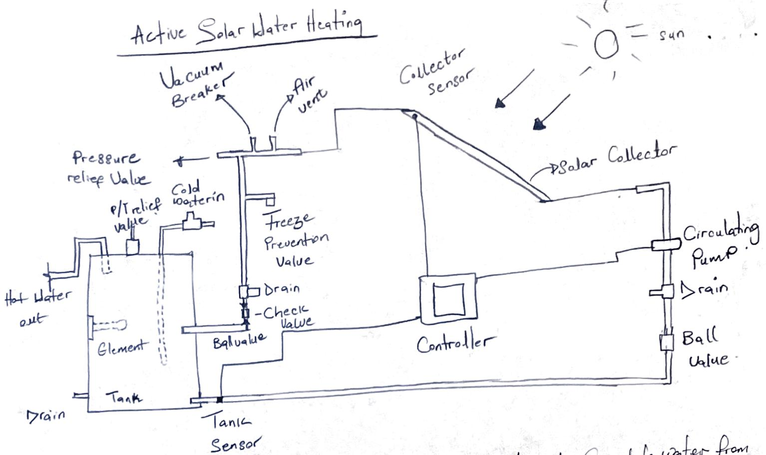
In an active solar water heating system pumps are used to circulate water from the storage tank to the collector with the use of ~~se~~ necessary elements. The active solar water heating system can be used through a direct system in which the water to be used would run directly through the solar collectors but in an indirect system water would run through the collectors then the heat exchanger to heat the water.
