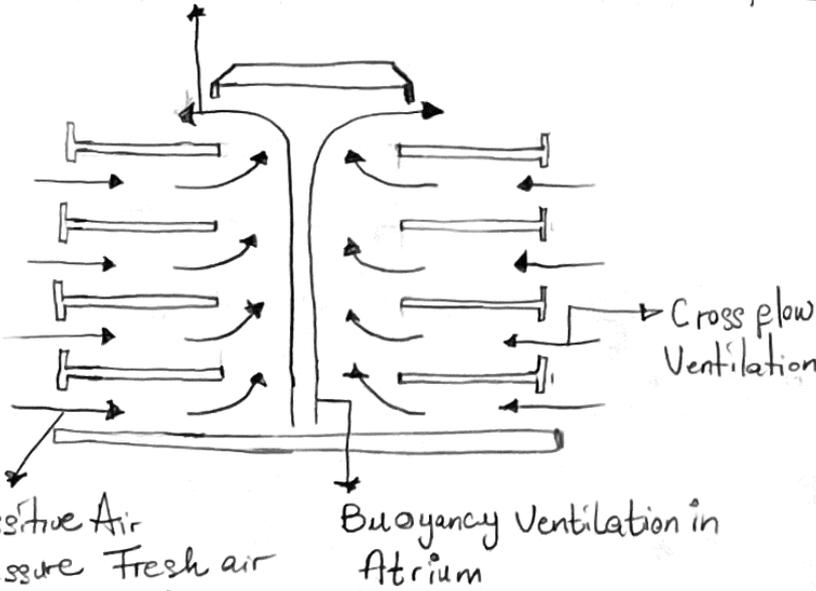
\* A Flow Diagram representing natural Ventilation through atria.
