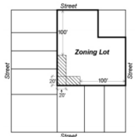
ZONING LOT BOUNDED BY TWO OR MORE STREETS (NEITHER A CORNER LOT NOR A THROUGH LOT) (33-261.2, 43-261.1)
