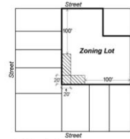
ZONING LOT BOUNDED BY TWO OR MORE STREETS (NEITHER A CORNER LOT NOR A THROUGH LOT) (33-261.2, 43-261.1)
