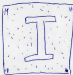
(E) Loose sheet insulating fill inside a metal enclosure
