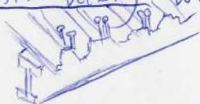
Cellular Decking - welding a corrugated sheet to form a series of splices or runways,
