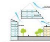
Stack Ventilation - Natural Ventilation
