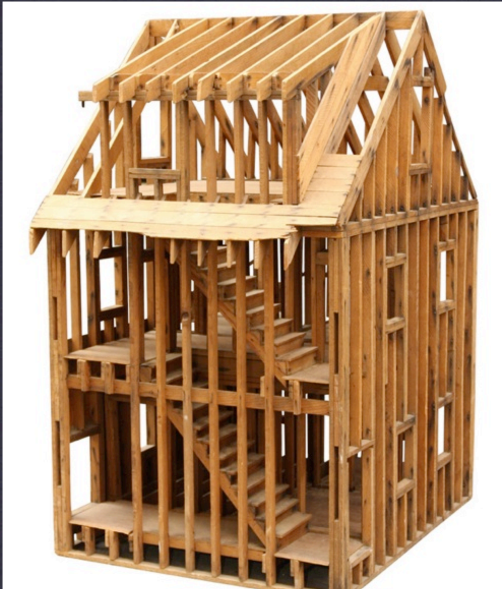
BALLOON FRAME CONSTRUCTION
