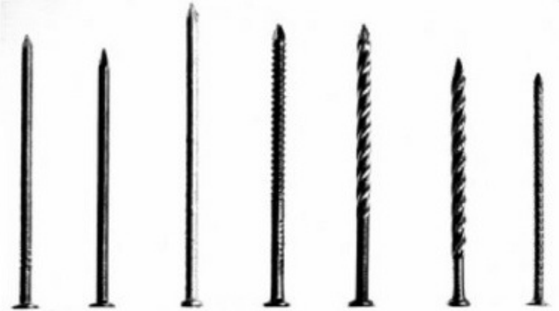
Various types of nails: (left to right) bright smooth wire nail, cement coated, zinc-coated, annularly threaded, helically threaded, helically threaded and barbed, and barbed.
