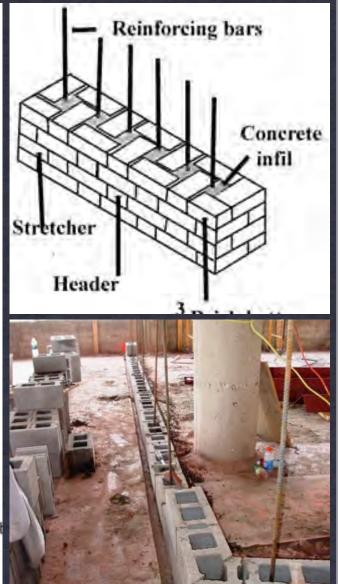
reinforced masonry walls
