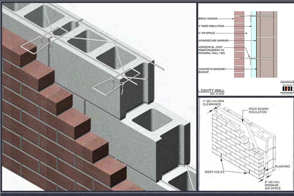
composite cavity masonry walls
