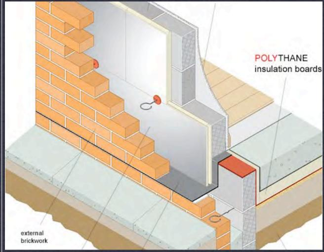
IMPROVED THERMAL PERFORMANCE: INSERT RIGID BOARD INSULATION INTO CAVITY W/ AT LEAST 1" AIRSPACE
