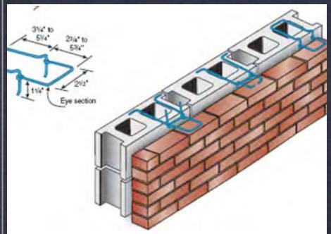
STEEL TIES CONNECT ACROSS THE CAVITY TO LINK THE INNER WYTHE OF CMU BLOCK W/ BRICK VENEER.
