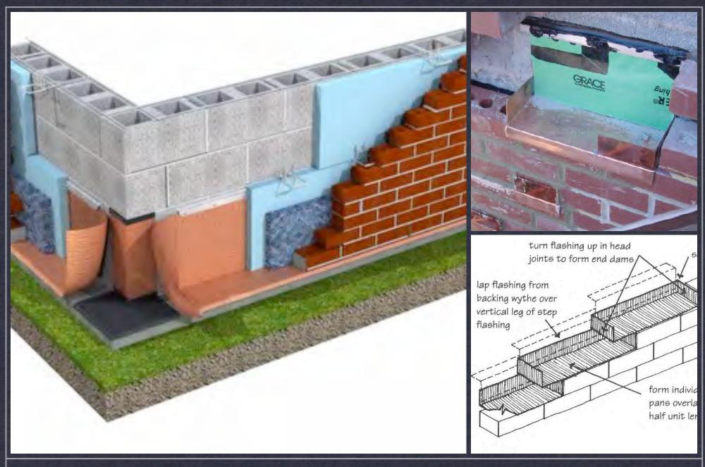
MASONRY WALL CONST. detailing: flashing @ exterior wall
