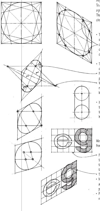
Any circles oblique to the picture plane appear as ellipses. To draw such a circle in a paraline drawing, we must first draw a paraline view of the square that circumscribes the circle. Then we can use either of two approaches to drawing the circle within the square.
