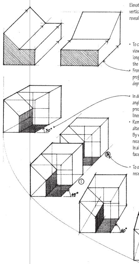
Elevation obliques orient a principal vertical face or set of vertical planes parallel to the picture plane and therefore reveal their true sizes, shapes, and proportions.
