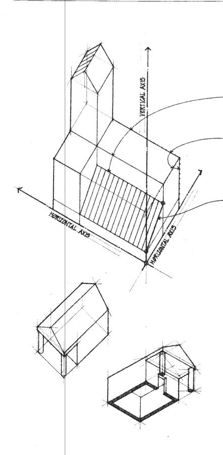
Paraline drawings communicate the three-dimensional nature of an object or spatial relationship in a single image. Hence, they are also called single-view drawings to distinguish them from the multiple and related views of plans, sections, and elevations. They can be distinguished from the other type of single-view drawing, linear perspective, by the following pictorial effects.
