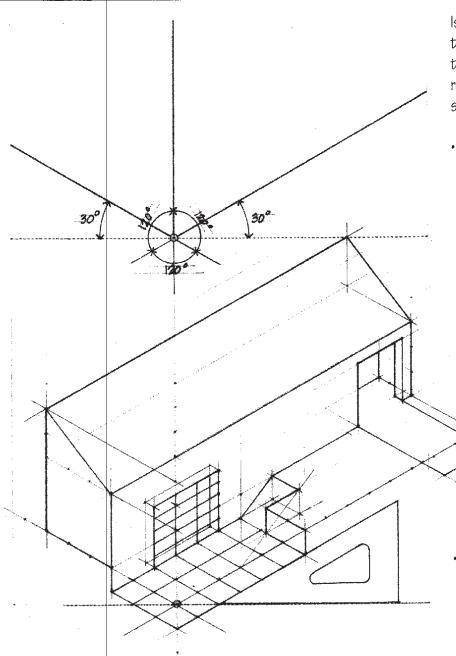
Isometric drawings establish a lower angle of view than plan obliques and give equal emphasis to the three principal sets of planes. They preserve the relative proportions of a subject or scene and are not subject to the distortion inherent in oblique views.
