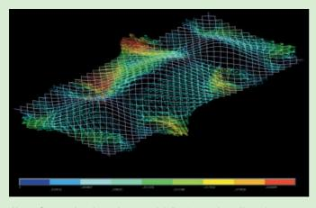
Above: Structural analysis of rotational deflections under self-weight. Below: Analysis of average daily insulation on roof panels without shading device (top) and with shading device (bottom).
