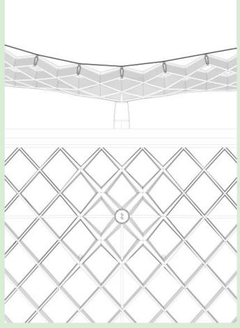
Elevation of column and section through roof beams (top) and reflected plan of column and roof beam connection (bottom).
