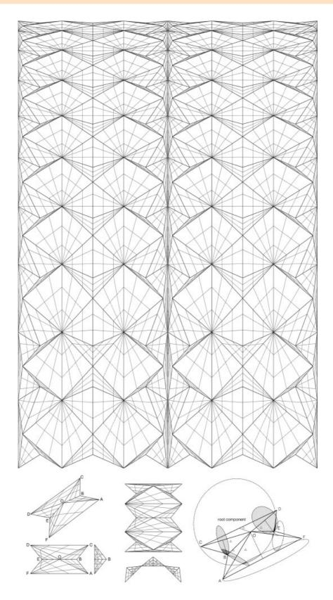
Parametric model of the folded generative component (bottom), and proliferation of component in one design solution (top).
