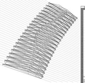
Parametric model of folded-plate roof project with spreadsheet of digitally derived geometric data.
