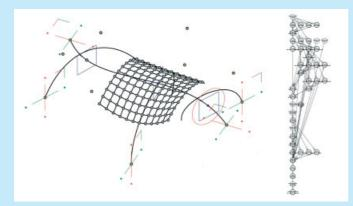
Figure 1 (left): Geometry model. Figure 2 (right): Symbolic model of the same parametric geometry of a double-curved surface.
