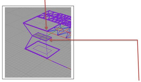
G. Run the slab command on each line, and choose a .125" offset and height. Make sure these offset towards the center of the model. This can be aided by snapping to the opposite corner of the platform when asked for the direction of the extrusion (for the line on the right this would be the top left corner of the platform).
