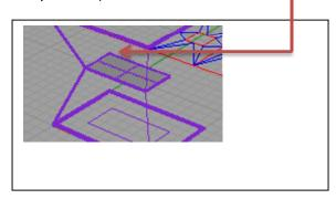
H. You can work with the Control Points of the diagonal line to adjust the slabbed form and minimize the needed trimming. If trimming is needed, trim the tops/sides of the connecting diagonal pieces as needed by creating a plane (*Cut Plane*) that will be used to trim with (NOTE: the plane needs to extend beyond the edges of the polysurface on all sides) and then running the trim command.
