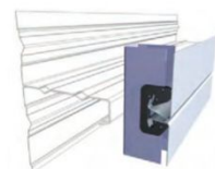
6. Modular click rail SE on structural cassette
