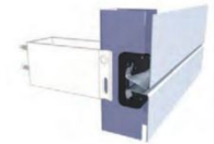
4. Modular click rail SE on U-brackets
