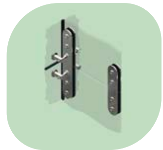
Vertical stainless steel splice plate connecting sections of a glass fin (mullion) together, incorporating Planar 905J fittings.
