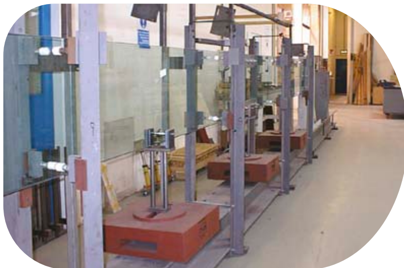
Glass Fin testing, Pilkington R&D Centre, UK.
