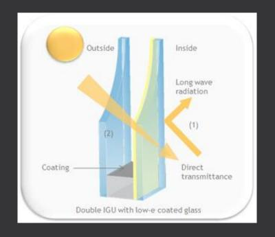
Pilkington Low-E 4th Surface Technology allows double-glazed insulated glass units to achieve better thermal performance. Applying two pyrolytic low-e lites in an insulated glass unit reduces the center-of-glass u-factor by 45%, compared to a unit with two panes of standard clear glass.
