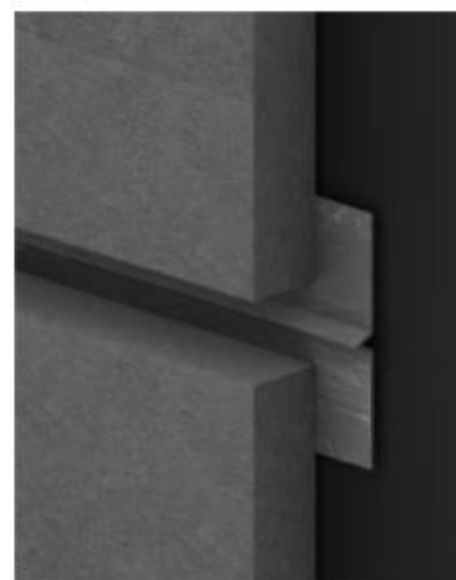
2) Closed joints where a horizontal joint profile is used to block the direct line through the joint.
