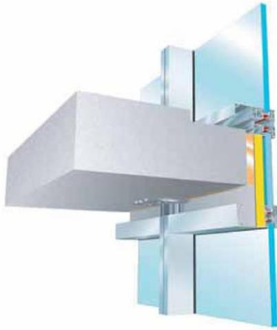
3D IMAGE OF SLAB EDGE ANCHOR DETAIL
