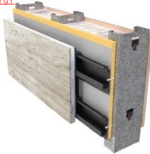
Figure 4 – Typical TerraCORE Panel Assembly
