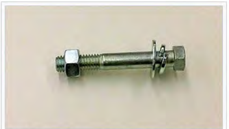
A plain washer and a spring washer are placed on a bolt between the nut (on the threaded end) and the bolt head.
