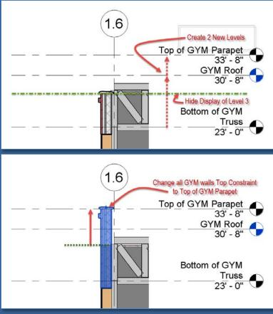
Select all GYM walls and change the "Top Constraint" to "Top of GYM Parapet"
