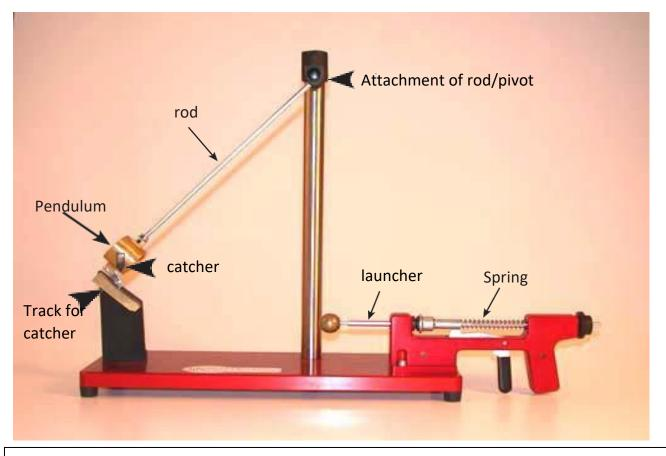
The above photograph shows the pendulum in the high position, prevented from falling by the "catcher mechanism". The launcher (marked h on the photograph) is in the extended state. The ball has been placed back onto the end of the launcher and this demonstrates the position of the ball immediately prior to leaving the launcher when it's shot. Compare with the photograph below to see the position of the pendulum prior to collision.
