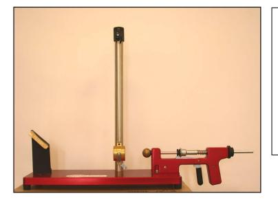
This photograph shows the spring loaded launcher compressed and ready to shoot the ball. But note that the ball is brought right up to the pendulum in the process of the launch so that the ball travels a distance on the order of 1cm or even less from the moment it leaves the launcher until the collision.
