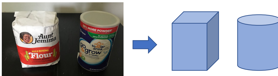
Fig.1 Example of two objects for the density determination (left) and their approximation as simple geometric shapes (right). In this lab, you use your own objects and their geometrical approximations. They should not be flour or a can – just use what you find in your room.
