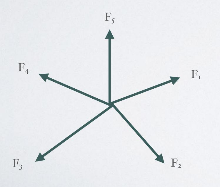
The free body diagram is a visual aid, to calculate the force vector use components
