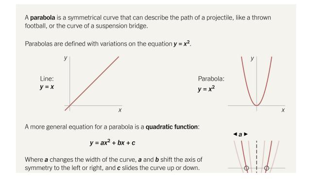
The **quadratic formula** learned by generations of math students is difficult to remember, but it can be used to solve **quadratic equations** where y = 0. Solving the equation gives the two points where the parabola crosses the x-axis (the two values of x when y = 0):
