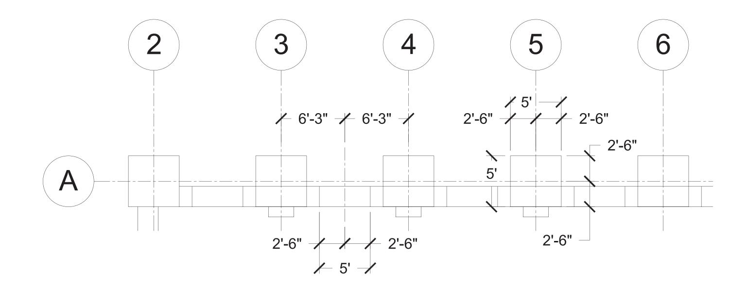
EXTERIOR WALL SETUP - USE YOUR GRIDS TO LOCATE EXTERIOR COLUMNS AND MAKE SURE TO CENTER WINDOWS
