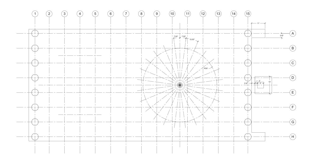
IDENTIFY KEY CENTERLINES AND LOCATE THE ROTUNDA - BEGIN LOCATING COLUMNS AT GRID INTERSECTIONS AND FINISH THE BASE
