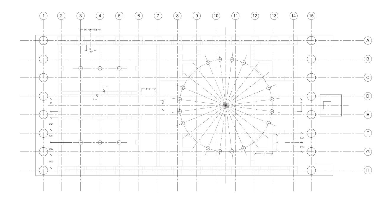
FINISH LAYING OUT INTERIOR PARTITIONS AND STRUCTURAL ELEMENTS, AND LOCATE DOOR AND WINDOW OPENINGS
