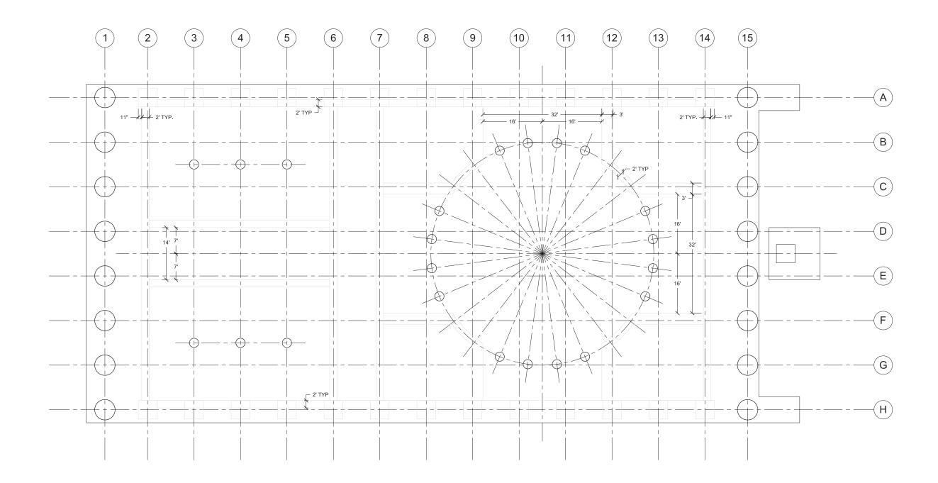
USING LIGHT CONSTRUCTION LINES, LOCATE INTERIOR AND EXTERIOR WALLS BASED ON DIMENSIONS GIVEN
