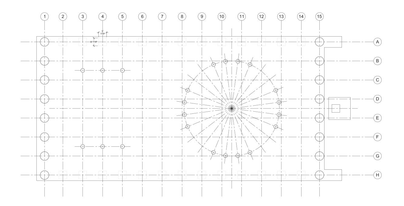
LAY OUT THE INTERIOR COLUMNS AND BEGIN SETTING UP THE 5'X5' COLUMNS AT THE EXTERIOR WALLS USING CONSTRUCTION LINES
