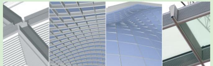
Digital detail of roof beam connection and gutter arrangement (left) of the roof structure (centre left); flat panel solution for glazing panels arrayed on double-curved roof surface (centre right); and related full-scale mock-up of roof beams and glazing built at the Gartner HQ in Gundelfingen, Germany (right).
