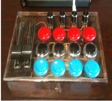
Controller send signals to Serial\_Midi converter
