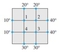
33. Write a system of four equations whose solution gives estimates for the temperatures  $T_1, \ldots, T_4$ .
