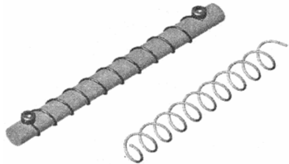
Figure 2: Example of a cylindrical mandrel – a shape-setting holding fixture to create helical springs [1].
